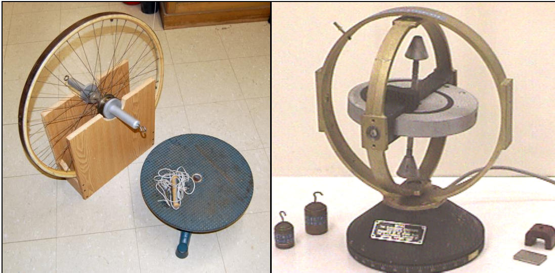
Figure 1. Altered bicycle wheel and turntable (left), gyroscope mounted inside double axis gimble (right)
