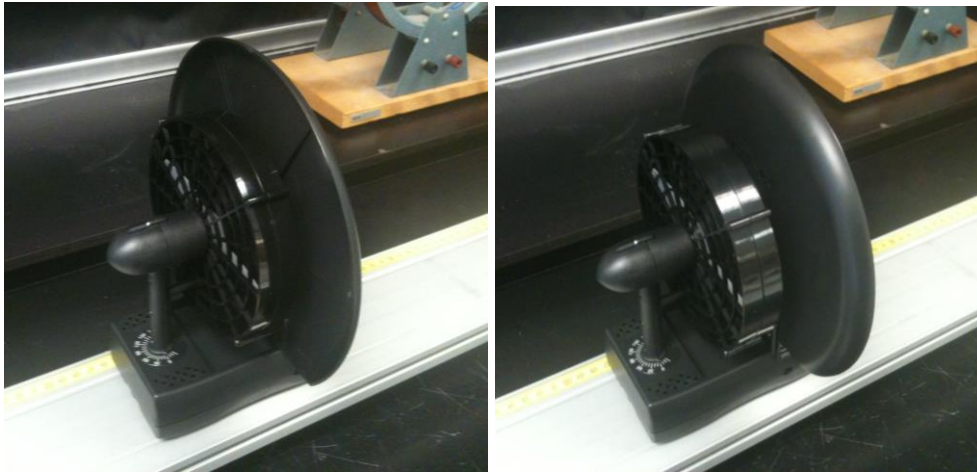
Figure 4. Left: sail attached forward, Right: sail attached backward
