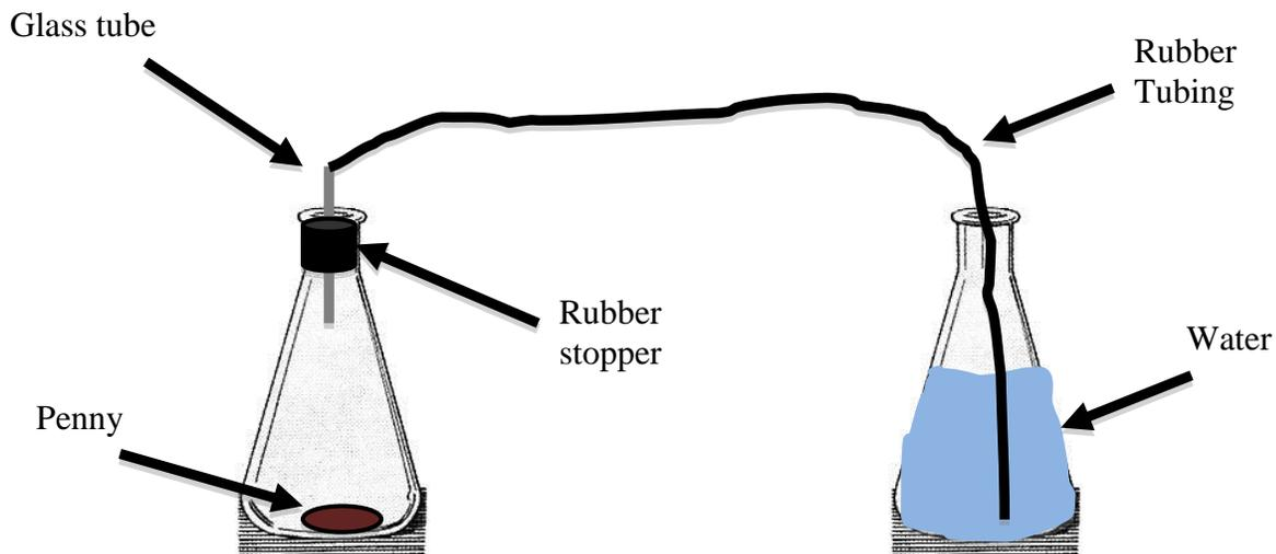
If you let the flask with the penny cool after the reaction, the reaction flask will draw water from the water flask and the solution produced will be a nice blue color. Also, to clean up, just put the reaction flask in the hood, and unstopper it with the fume hood on. Then, pour water into the reaction flask.
